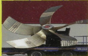
5-blade 4.3m fishing propeller
