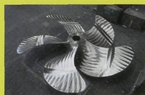
5-blade high skew coasting propeller
