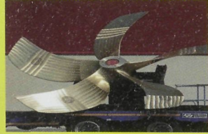
5-blade 4.3m fishing propeller
