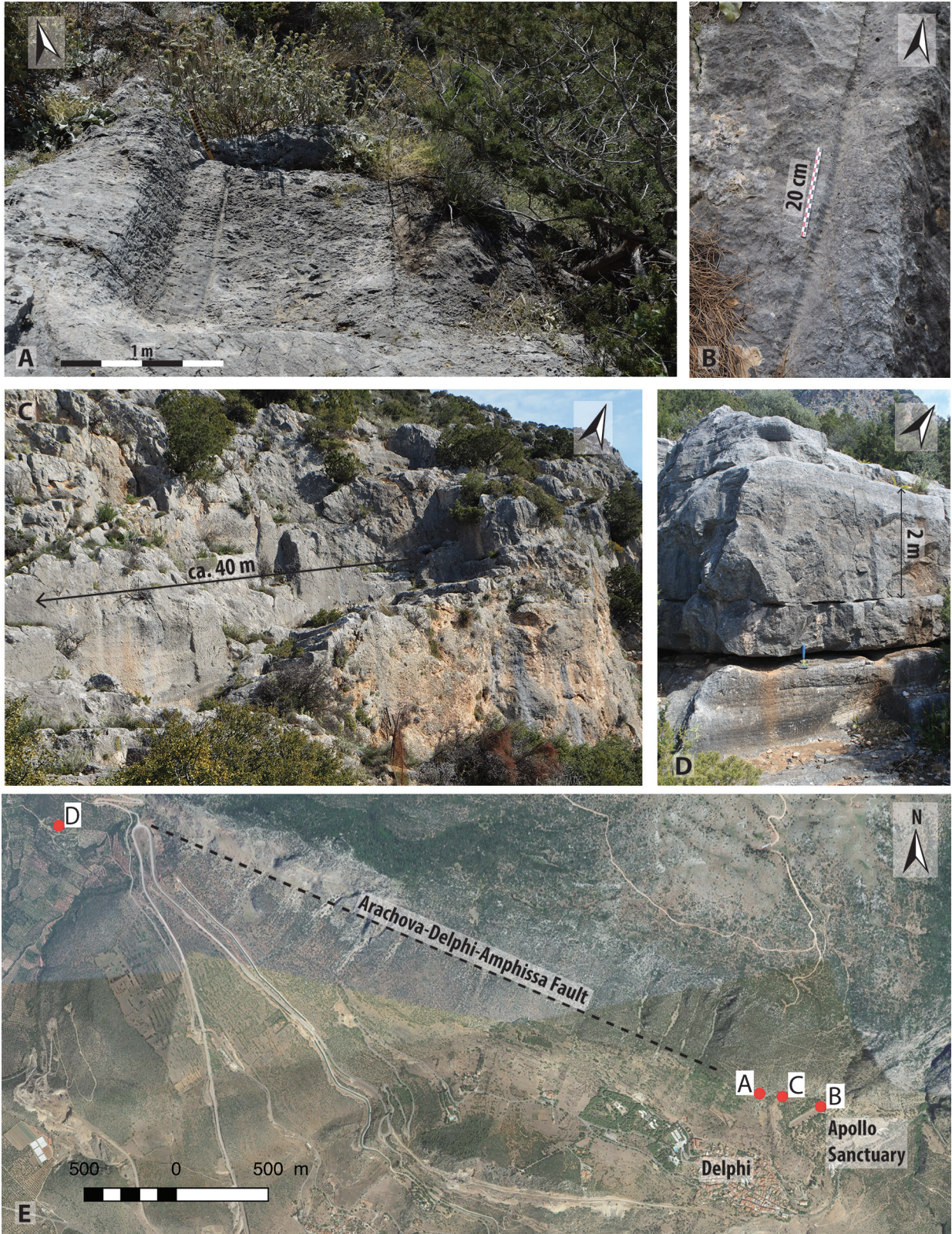
Fig. 10. A local exploitation. A. Extraction marks observed at the top of a rock that fell of the cliff above Delphi. B. Extraction tool mark observed at the foot of the main fault, hundred meters west of the Apollo Sanctuary. C. Stadium Quarry, located just above the stadium. D. The ancient Profitis Ilias quarries, 5 km west of Delphi. E. Location of the extraction sites.
