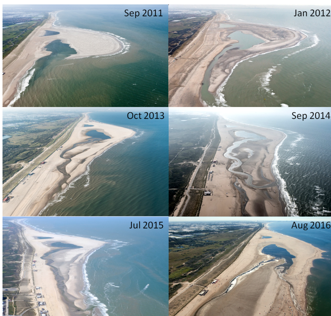
Figure 1. Aerial photographs of the Sand Engine in the period 2011–2016, looking south. Photographs courtesy of Rijkswaterstaat/Joop van Houdt and Jurriaan Brobbel, available through: www.flickr.com/photos/zandmotor .
