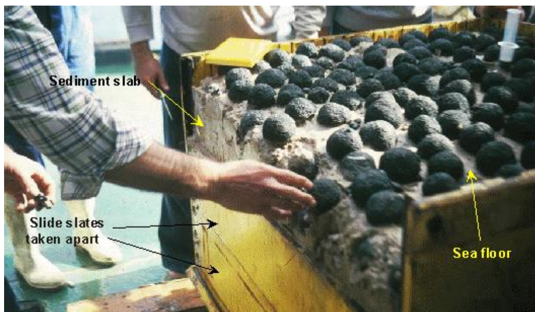
Figure 16. Nodules and mud in a box corer (SYMPAS). Source: Museum National d'Histoire Naturelle [61].
