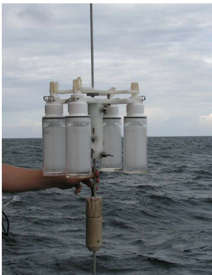
Figure 2. Modified MERCOS water sampler of the first (above) and second generation (below) for four bottles, manufactured by BSH, Germany (photos by courtesy of M. Haarich, vTI, and S. Schmolke, BSH, Germany).
