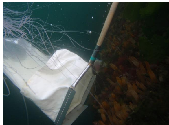
Figure 2.7: A handheld scrape with pocket net was used to collect samples from submerged infrastructure. Photo: Marte Svorkmo Espelien
