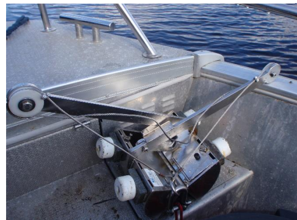
Figure 2.6: Bottom sediments with infauna was collected with a hand operated grab. Photo: Marte Svorkmo Espelien
