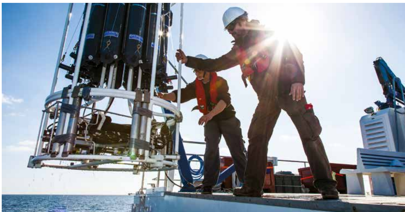
Deploying a Conductivity, Temperature and Depth (CTD) profile and water sampling bottles (-rosette), one of the basic equipment capabilities, from RV SOCIB.
