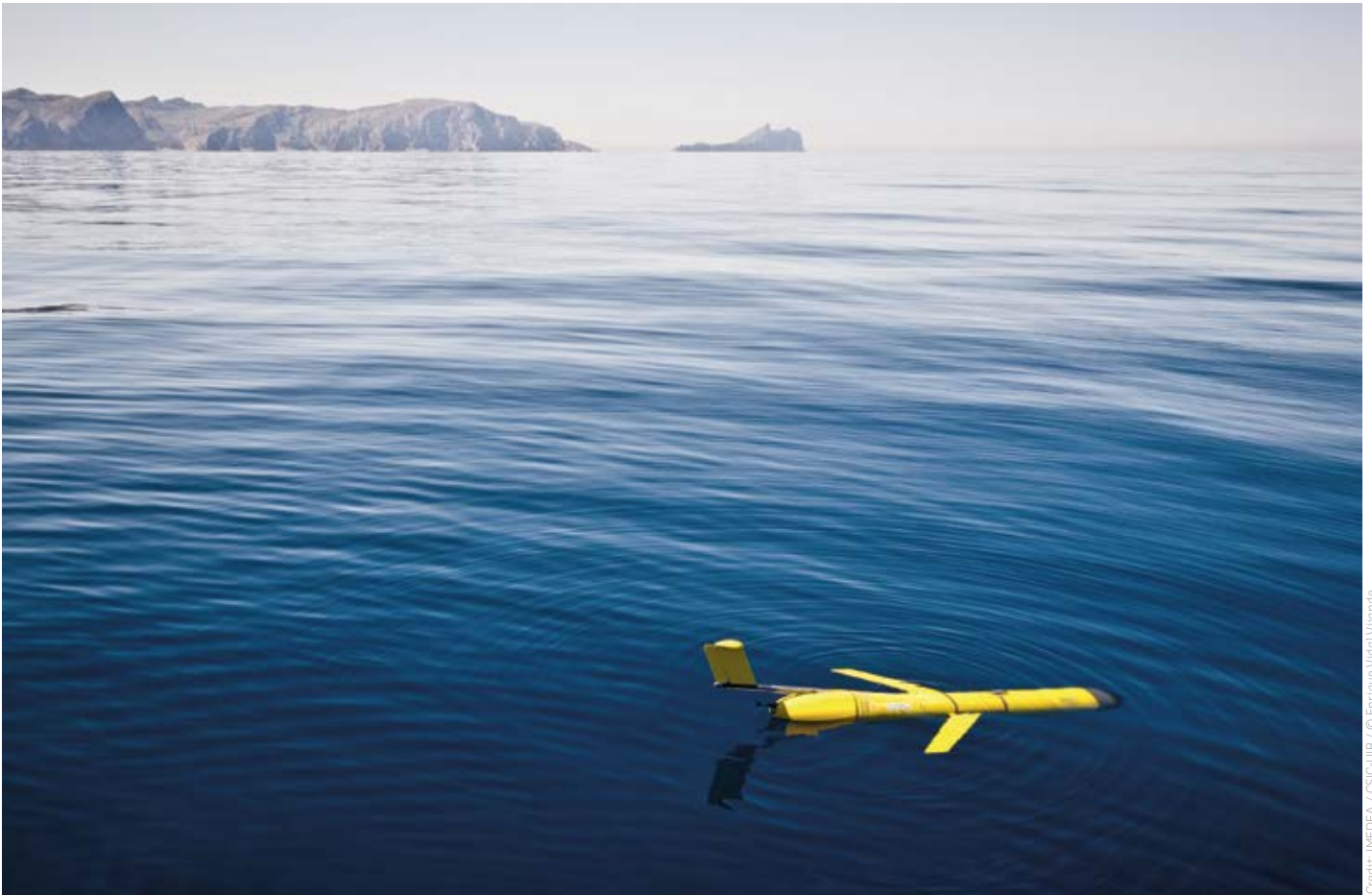
A Slocum Glider floats on the sea surface transmitting mission and sea state data via satellite to the IMEDEA (Mediterranean Institute for Advanced Studies) data facility.
