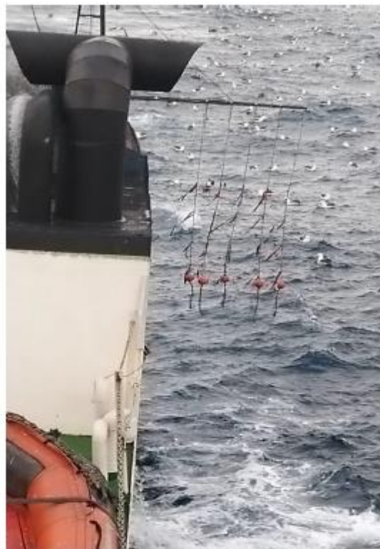
Figure 2. System of "tangones" with ropes on trawler Factory vessel.
