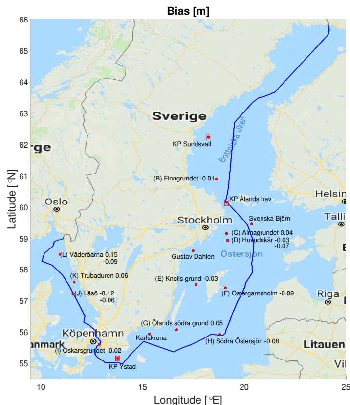
Figure 2. Map of the SEEZ with 17 selected grid points (marked in red) with saved full two-dimensional wave spectral information. The numbers at the 14 buoy locations denote the bias (Table 2). Locations marked with red squares (KP Sundsvall, KP Ålands hav, KP Ystad) had no wave buoy measurements but the two-dimensional wave spectra were saved. A dark blue line is included to indicate the extent of the SEEZ.
