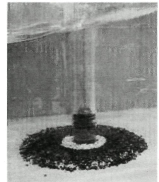
Figure 2. Experimental set-up: scour protection on a sand bed around monopile.
