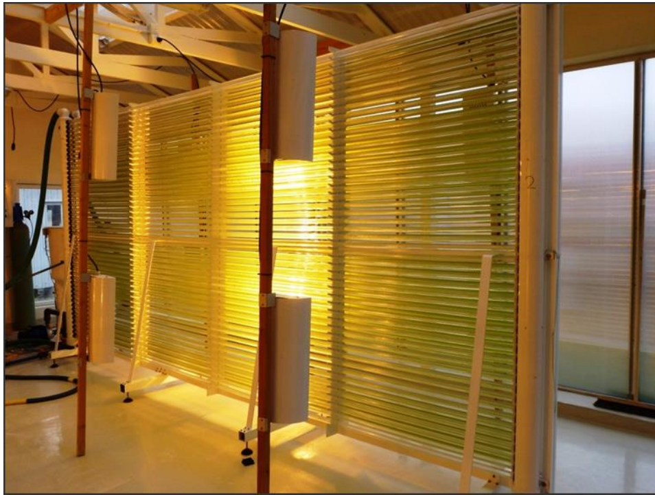
Figure 22: Mass production of microalgae in a photobioreactor system (Biofence).
