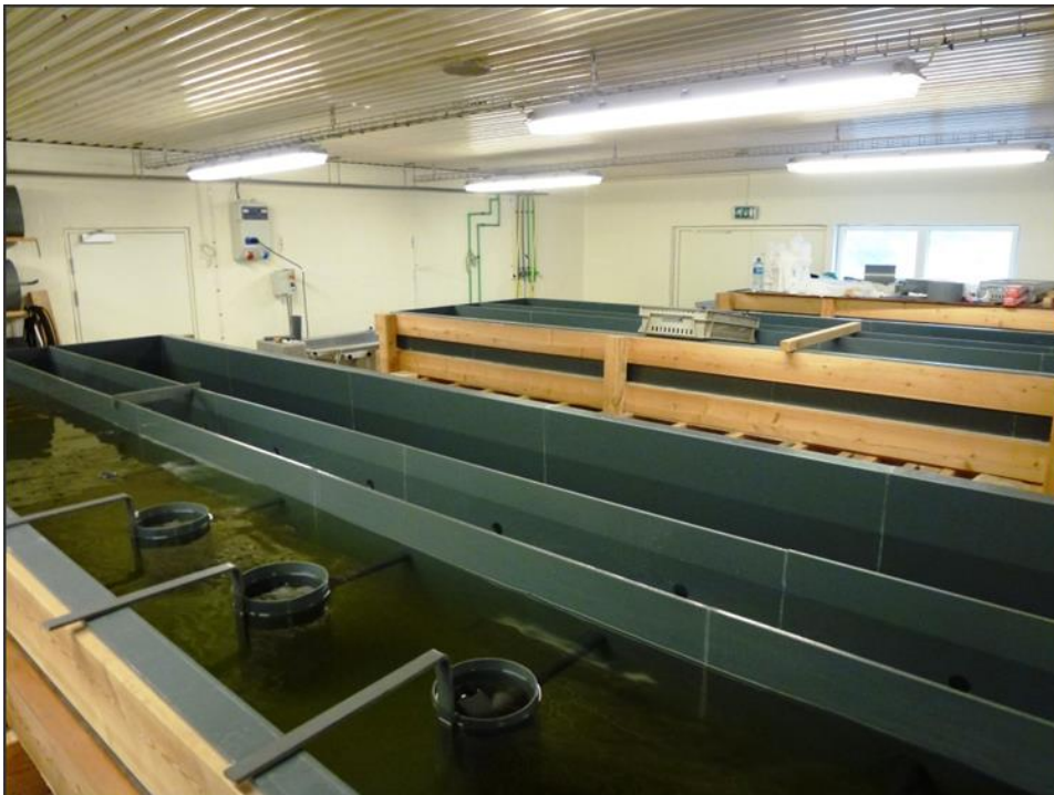
Figure 25: Hall for growing spat. Early stages of spat are located in the round containers that are immersed in the trough-shaped tank.
