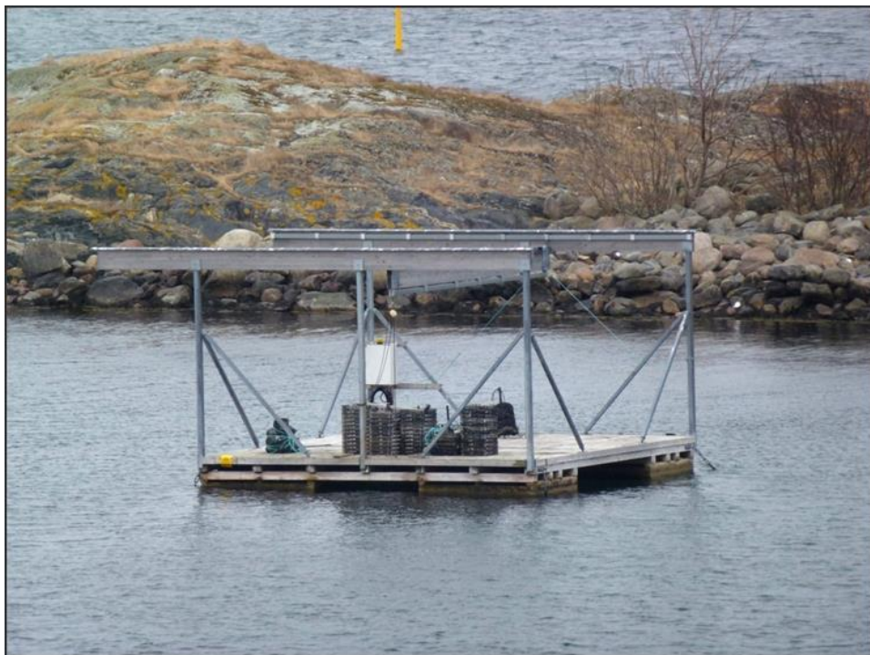
Figure 27: Hanging baskets with spat on the raft. The FLUPSY system ensures a constant supply of water and therefore also of food.
