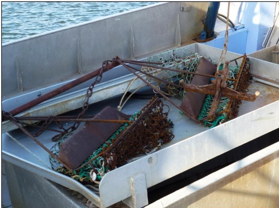
Figure 37: For the oyster harvest, the use of smaller and lighter dredges (max. 35 kg) is mandated.
