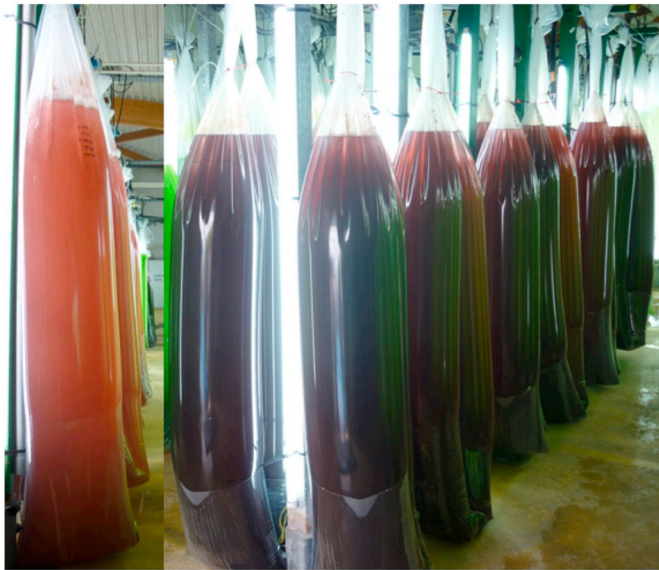
Fig. 8. Culture of Porphyridium cruentum in polyethylene sleeves (Greensea, Mèze, France).
