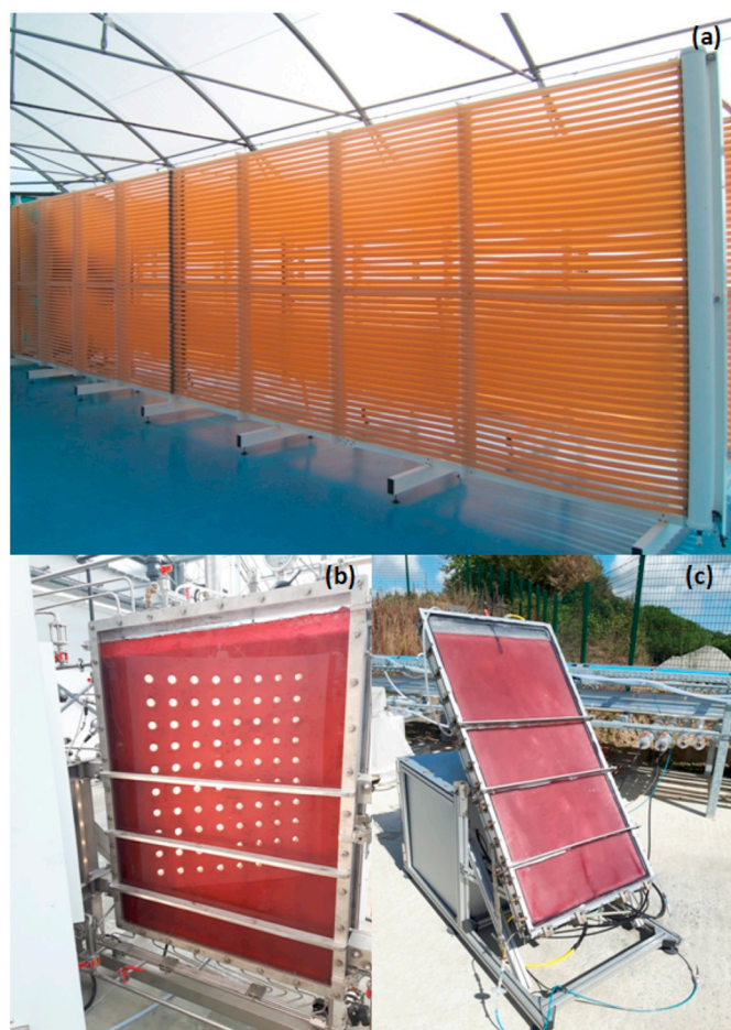
Fig. 10. Cultures in different photobioreactors from different companies. (a) Porphyridium cruentum , vertical tubular photobioreactor (Greensea, Mèze, France); (b) Porphyridium cruentum , flat plate photobioreactor with artificial light and (c) Porphyridium cruentum , inclined flat plate photobioreactor with natural light (AlgoSolis, GEPEA, Université de Nantes, CNRS, France).
