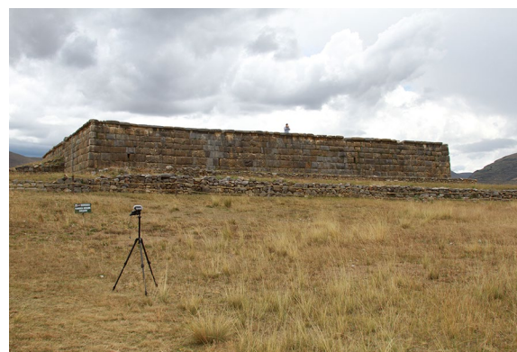
Fig. 1 Acoustical survey around the central platform at Huánuco Pampa: one of five sound sources used in the survey, a Strombus pututu (conch horn), performed from eastern platform-top niche (survey point “S2”); recorded using tripod-mounted audio recorder with GPS device on plaza ground; sound-level metering and photo/video documentation equipment not shown
