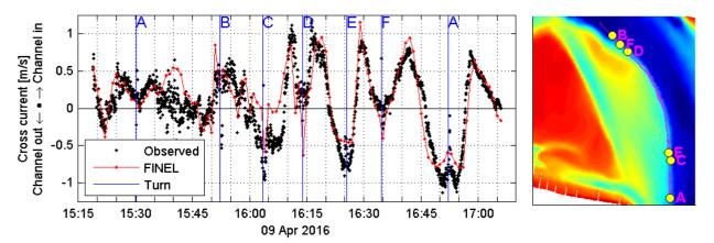
Observed and modelled cross current in the navigation channel near Ossenisse. Note that the observations are sailed current measurement, and the location of the vessel varies in time. The moments the vessel turns around and the vessel track are indicated as well.
