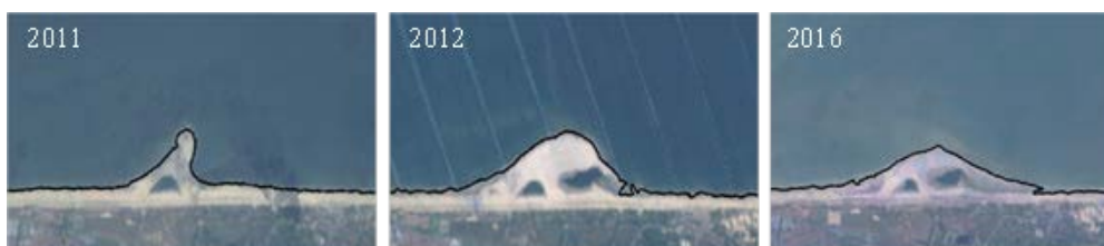
Figure 1: Evolution of the SDW position (black line) for the Sand Motor study area. From left to right: construction of the Sand Motor in 2011, the situation in 2012 and the present state in 2016.
