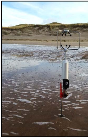
Figure 1: Ultrasonic anemometer installed, as a part of a cross-shore array, at the beach south of Egmond aan Zee. The tall and steep foredune front is visible in the background.
