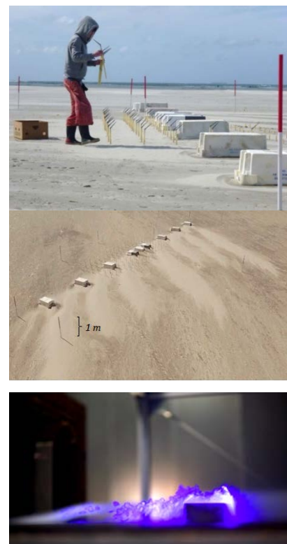
Figure 1: Impression of flow visualization experiments around scaled beach house on Terschelling beach and in the wind tunnel of the department of Engineering Fluid
