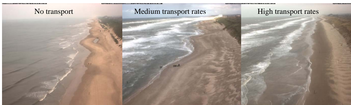
Examples of ARGUS photos showing no, medium and high amounts of sand transport. Source: ARGUS Coast3D tower.
