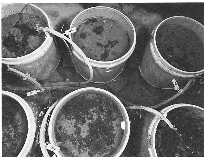
Boxcosms with manipulated North Sea sediments: upper series (43/44) with macrofauna, lower series (39) without macrofauna, several days after an organic matter supply. (Photo: NIOZ)
