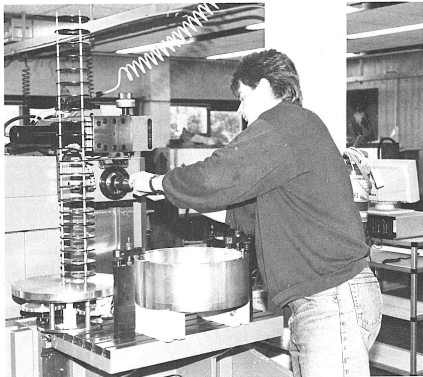
The 22 channel transmission meter under construction at the NIOZ instrumental department. (Photo: NIOZ)
