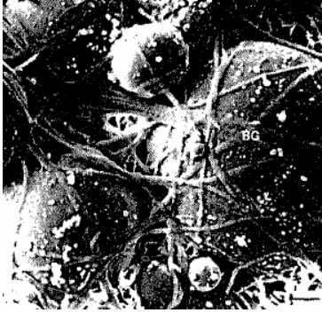
Figure 8. SEM image showing adhesive bonding of glass beads by polymeric strings (Paterson, 1997). The average size of the beads is around 50 \mu\text{m} .
