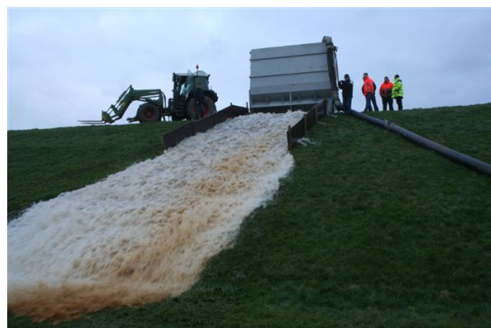
Fig. 2. Investigating grass performance under overtopping
