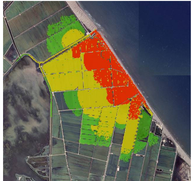
Fig. 2. Example of different flood extents generated based on different definitions of the coastline (North Ebro delta coast)
