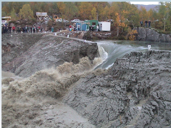
Fig 1. Breach field test (IMPACT project)
