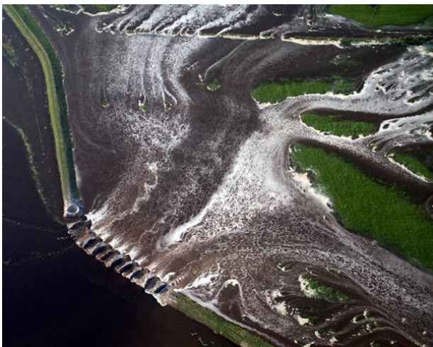
Fig. 2. Aerial view of a polder breach on the River Elbe (courtesy of Zebisch)
