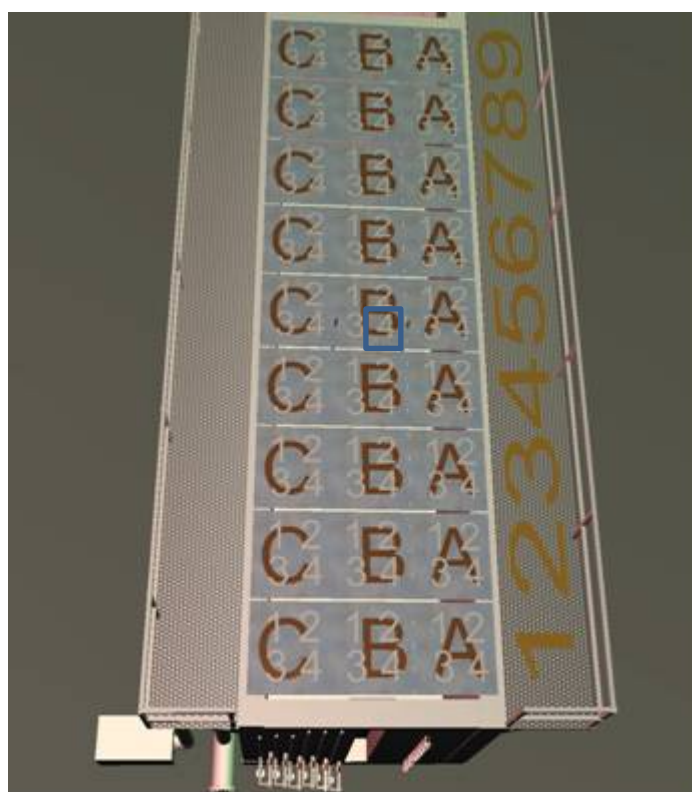
Figure 2: Test tank compartments of the sediment test tank –top view. The blue box represents the 5B4th position: 5 is the location of the bridge (vertical numbering: 1-9) and B is the position on the bridge. In the B (horizontal numbering: C-B-A) position 4
