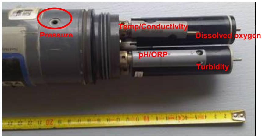
Figure 7: Pressure probe and different sensors inserted in the multi-parameter probe '6920V2-M'
