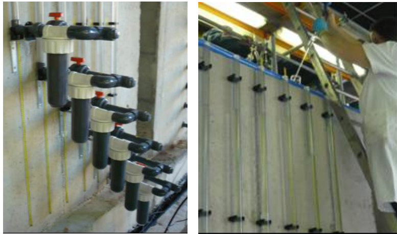
Figure 5: Piezometric tubes and filters (left) were immediately filled up with water after filling up the tank (right)
