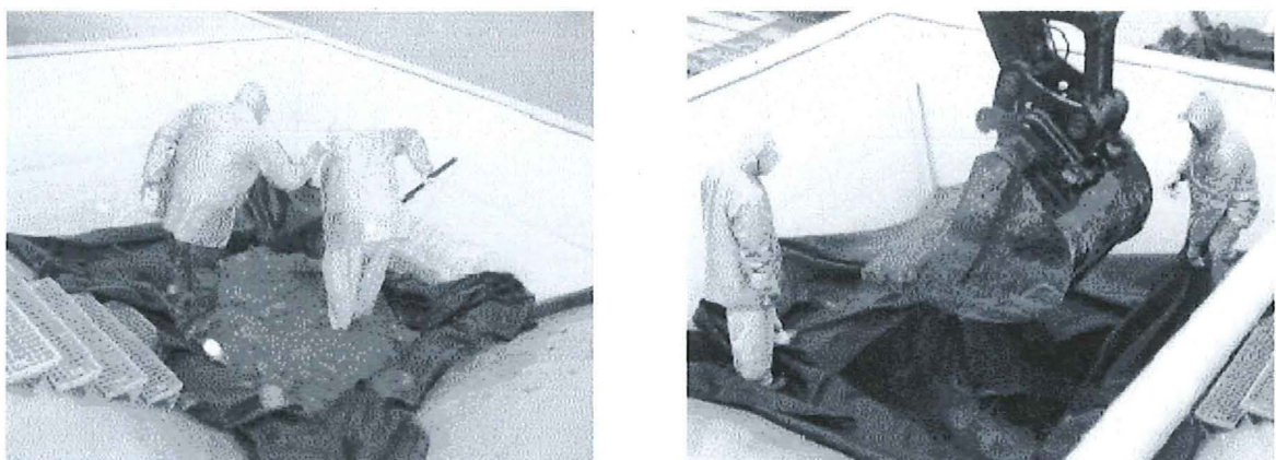
Figure 4: Picture of filling of the mesocosm with both soils. First, water permeable plastic was placed to avoid that soil would leak out of the mesocosm.
