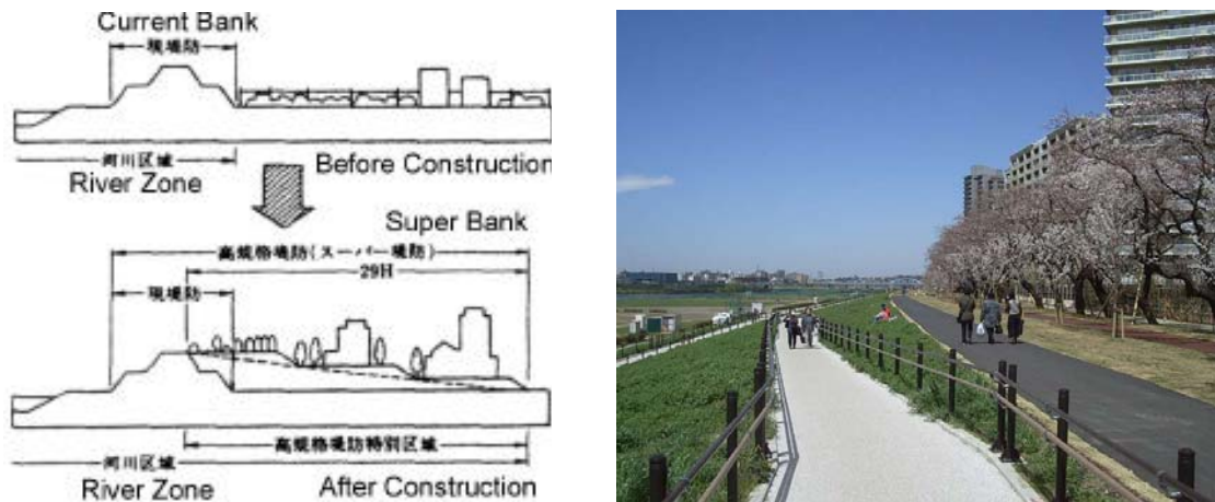
Figure 3 – Example of a super dike along Yoko River, Japan (L: BTL Committee, 1998; R: Deltacommission, 2008)
