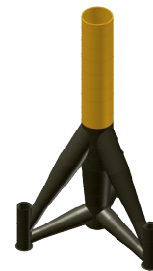
Figure 7 – Tripod foundation used at Park Alpha Ventus [2]
