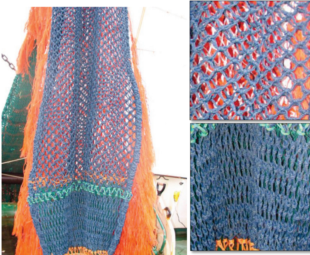
FIGURE 2-1 – T90 COD-END WITH A POSTERIOR SHEET OF NETTING (5 ROWS) WITH T0 ORIENTATION (LEFT) - T90 (TOP) AND DIAMOND MESH NETTING (RIGHT)
