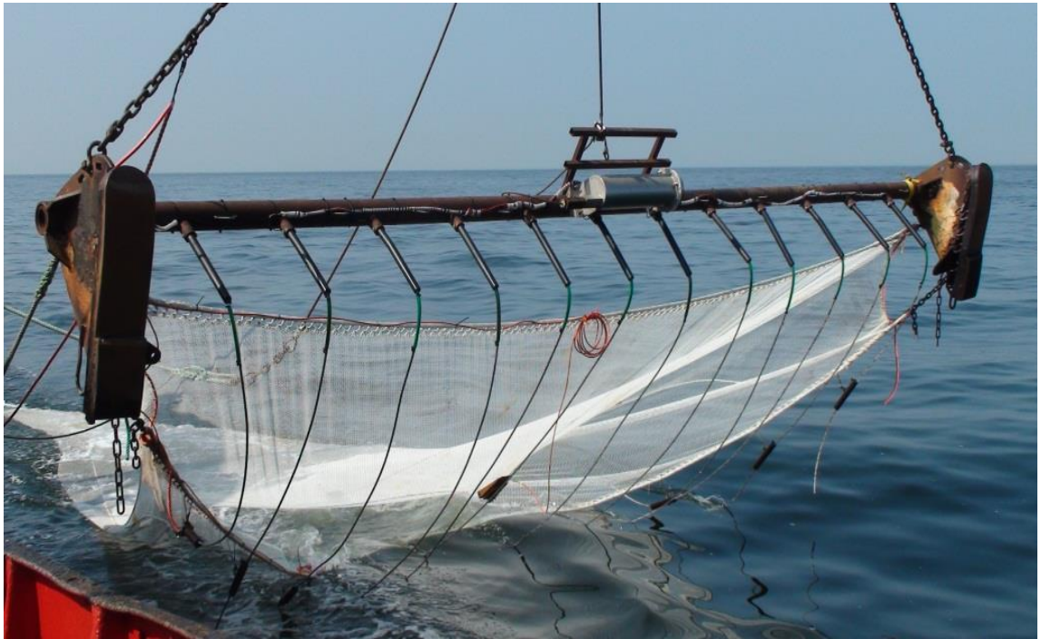
Figure 1.3: The Hovercran with 8 m beam and trawl shoes. The cylinder fixed on the middle of the beam is the pulse generator.
