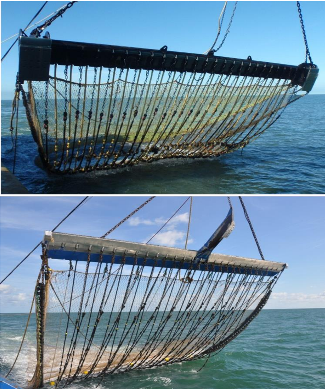
Figure 1.1: The Delmeco pulse beam with beam and trawl shoes (A) and the HFK Pulse Wing with the wing and the runner in the centre (B).
