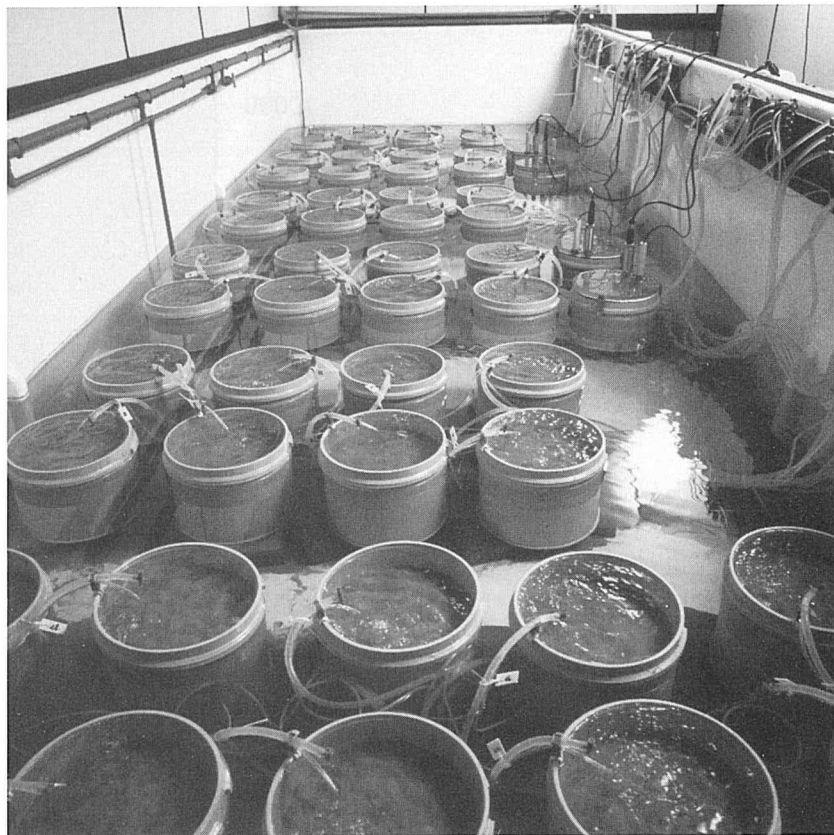
The North Sea boxcosm experimental set-up. Oxygen consumption measurements are taken on the rear right-hand side. (Photo: F.C. van Duyl)
