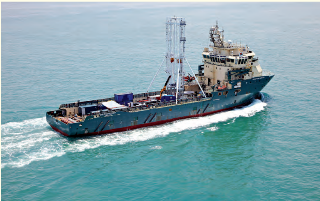
Figure 4.3. The Greatship Manisha, drillship of IODP Expedition 347 is equipped with the drill rig Geoequip Marine's GMTR 120 Geotechnical and Coring Rig (photo Geoequip Marine, courtesy of Island Drilling Singapore Pte.Ltd).
