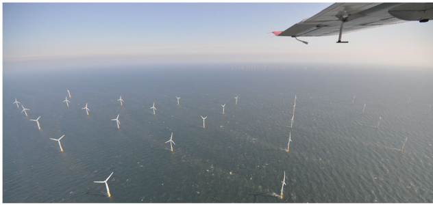
Fig. 1 Aerial photograph (SE view perspective) of the Belwind OWF (southern North Sea) on 18th March 2014 (01.30 p.m. UTC, altitude about 500 ft, RBINS-OD Nature flight), showing SPM plumes in the wakes of the turbine piles around maximal flood current at spring tide (full moon phase). Photograph taken by MUMM, RBINS-OD Nature
