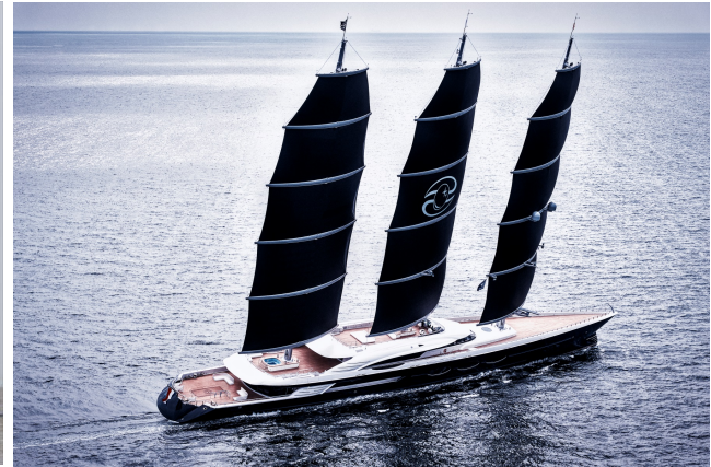
(a) The E-Ship 1, manufactured by Enercon and equipped with 4 Flettner rotors [57]. (b) Oceanco's Black Pearl, incorporating modern square rigs [58].
