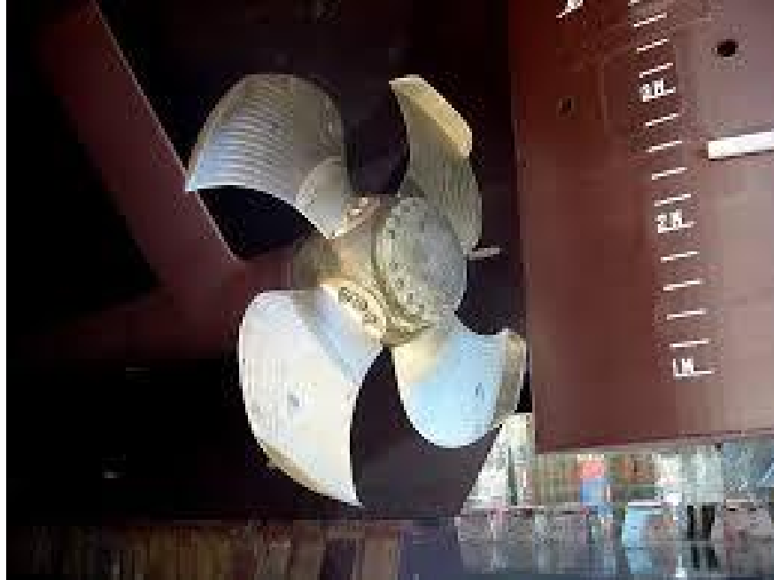
Figure 11. A contracted and loaded tip propeller [36].
