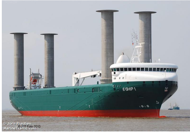
(a) The E-Ship 1, manufactured by Enercon and equipped with 4 Flettner rotors [57]. (b) Oceanco's Black Pearl, incorporating modern square rigs [58].
