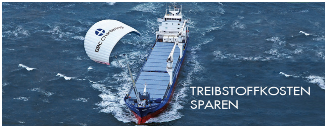
Figure 16. Towing kite SkySails [52].
