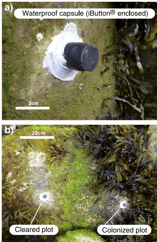
Fig. 2. Deployment of temperature loggers encased in waterproof capsules (a) on a concrete pylon in Newlyn Harbour and (b) limestone rock rubble at Portland Port.
