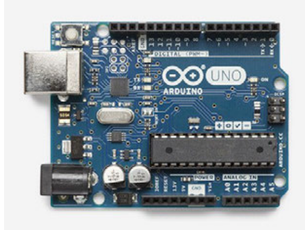
Figuur 17 Arduino Uno board Bron: Arduino [9]
