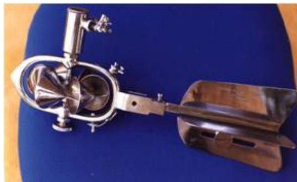
Figuur 12 Cup-type rotor Bron: Cwprs [19]
