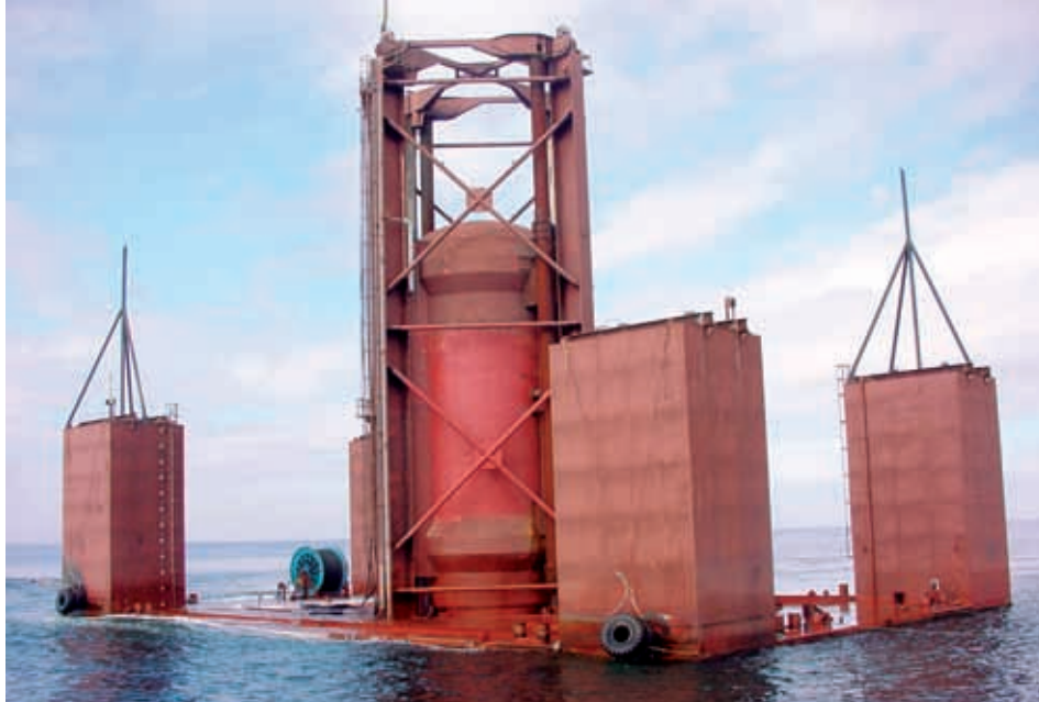
■ Archimedes Wave Swing: pilootproject met 2MW prototype (AWS ocean energy TLD)
