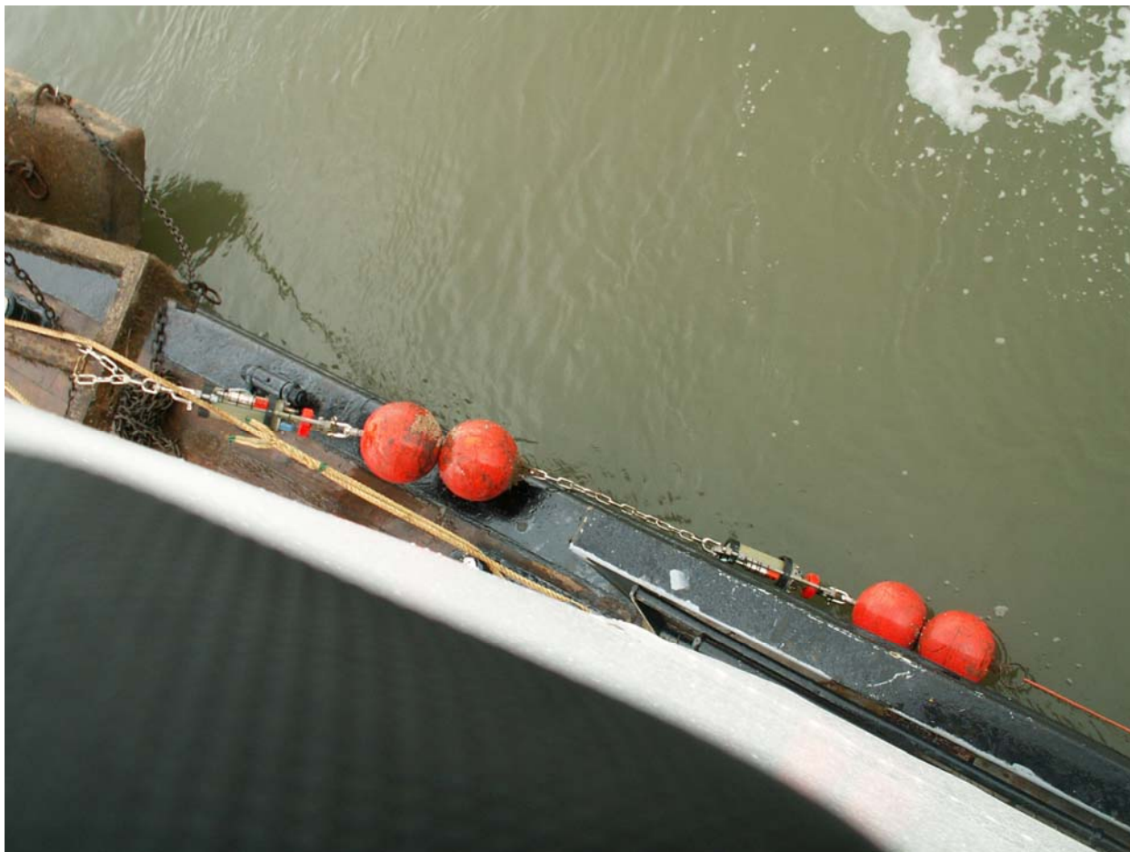
Figure 3-18: Set-up of two RCM-9 units
