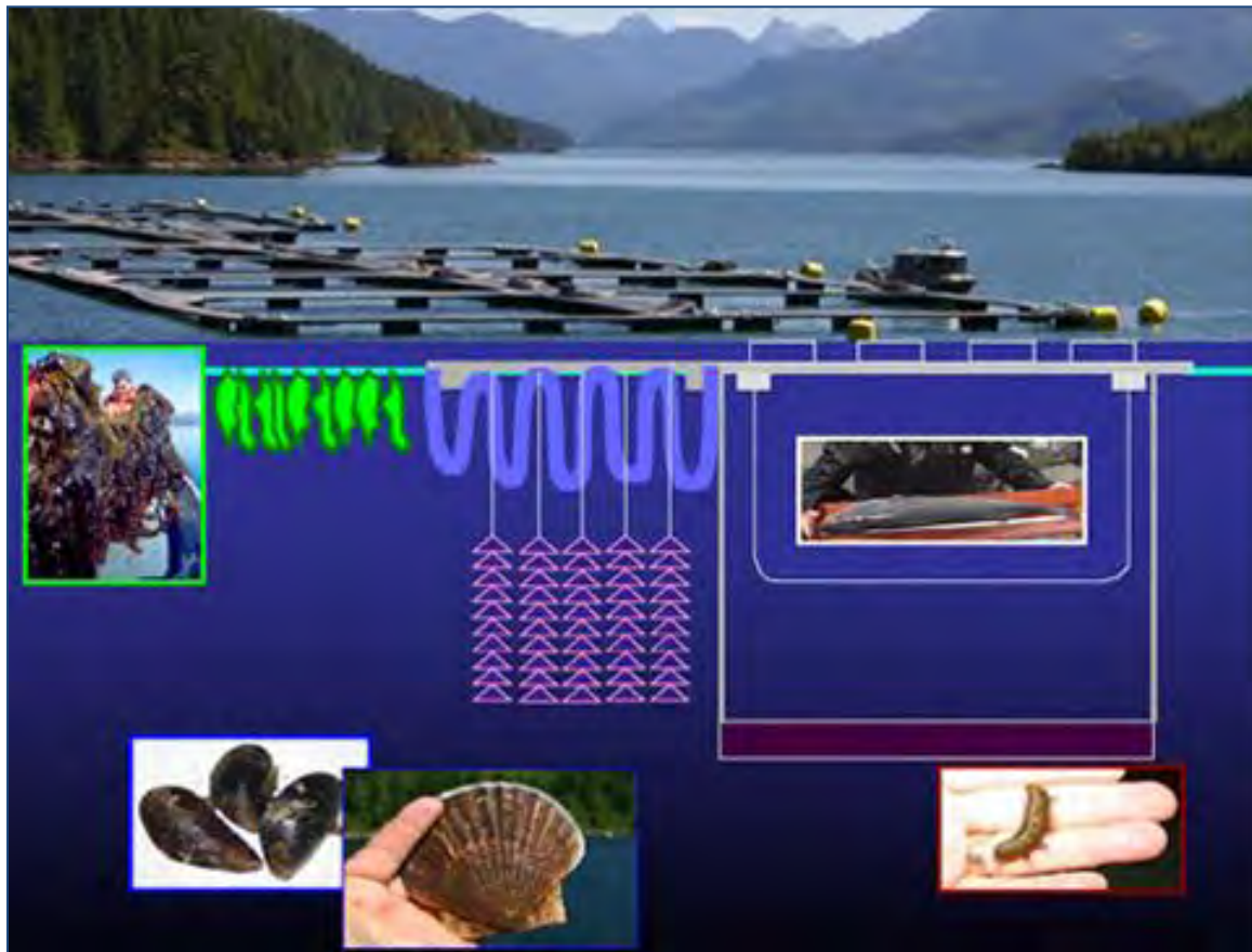
Fig. 10-42 - A diagram of an IMTA system, showing the interlinked ecosystems under the water. The bright green areas on the left-hand side are kelp; the wavy blue lines are mussels; the pink triangles are shellfish; the main cages contain salmon, and the bottom purple 'strip' contains sea cucumbers, which feed on more solid waste.
