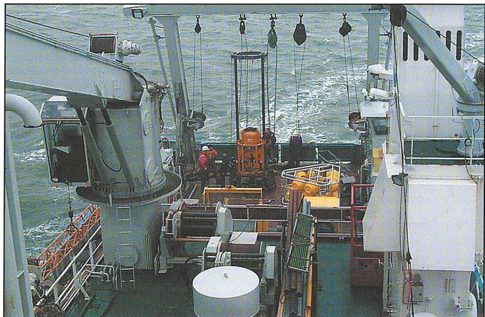
Testing the vibrocorer Drammensfjord 1 November 1999. (photo: Jack Schilling)
