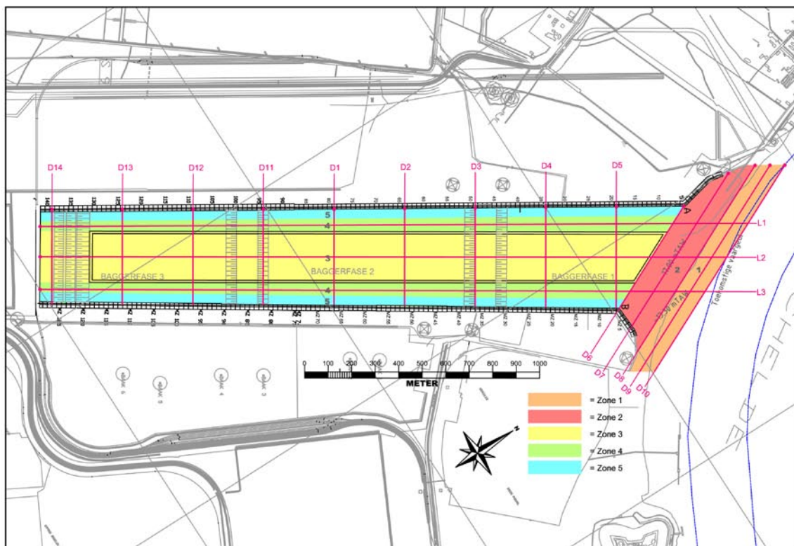
Figure 4-2: Deurganckdok: D and L Sections
