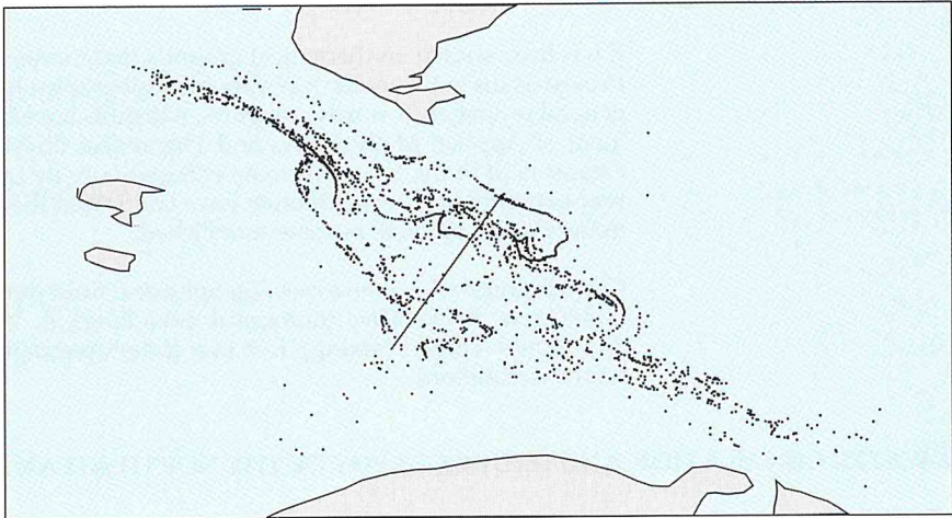
Depicted is the chaotic advection of a line of 1000 particles, indicating rapid mixing of the tidal area. These particles were initially released in an eddy located in the tidal channel of the Ems estuary, a shallow tidal area in the eastern Dutch Wadden Sea and are shown after 0, 1, 2, 3 and 4 tidal periods.
