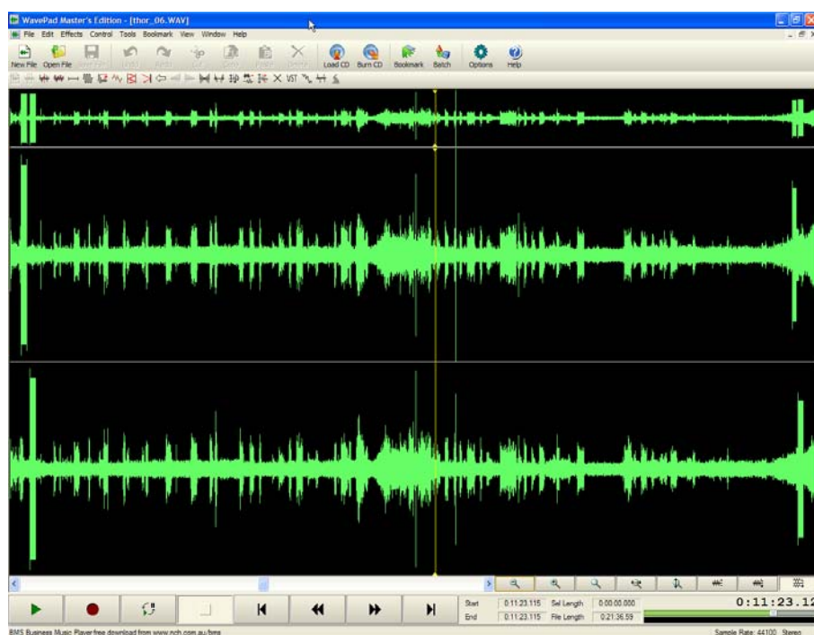
Figure 7. Raw data file Thor_06.wav, 10 September 2008. Middle graph: underwater noise level, upper hydrophone; lower graph: underwater noise level, lower hydrophone; the top graph is the sum of the two other graphs.
