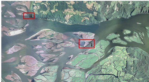
Figure 1. The Columbia River Estuary, WA, USA. Well-developed bar complexes can be seen throughout the channel, some of which are vegetated. Data on two bars are presented herein: i. Sandee Bar, where ADCP measurements were carried out (Figs 2 and 3); and ii. Wills Bar where the MBES survey shown in Figure 4 was conducted.
