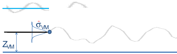
Figure 4. Vertical ship motion above horizontal bottom
