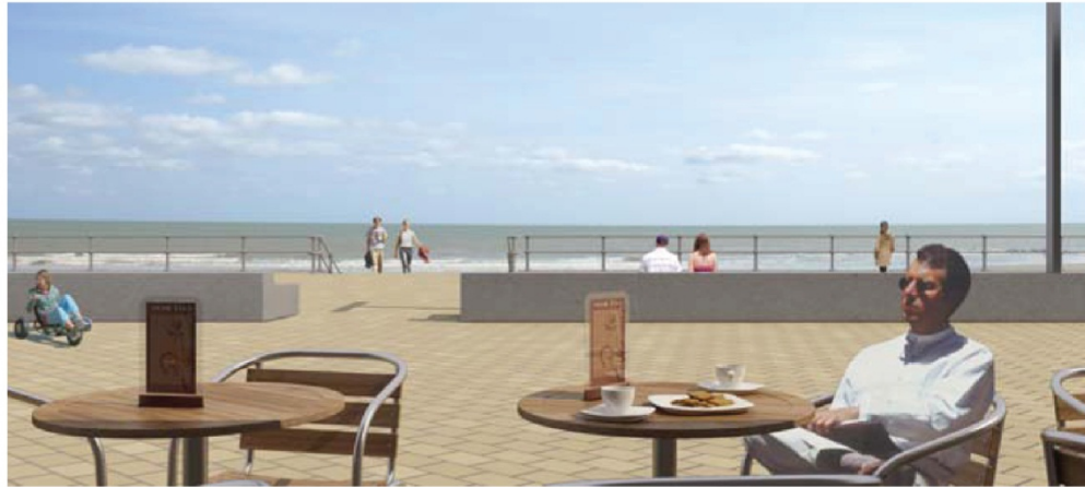
The dyke reinforcement of 60cm can be disguised as a concrete bench. ... (Masterplan Coastal Safety Flanders, 2012)
