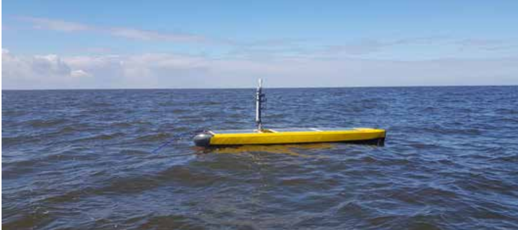
The Unmanned Surface Vehicle (USV) 'Adhemar' is energy neutral and can stay at sea for weeks or months on end.
