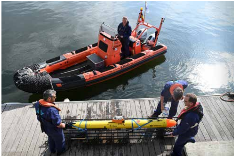
Scientists and technicians demonstrated the operation of the autonomous underwater vehicle (AUV) Barabas during the press presentation of the Marine Robotics Centre. © VLIZ (Verhaeghe)
