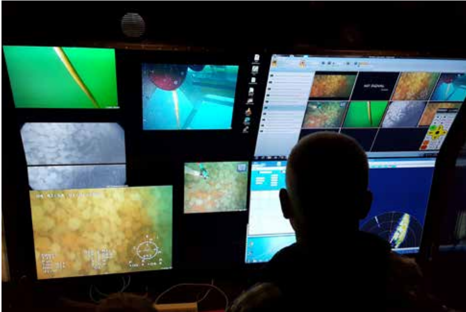
The activities of the remotely operated underwater vehicle Genesis are closely monitored in the control room. © VLIZ
