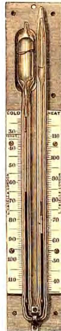
FIG. 53.—The Miller-Casella modification of Six's self-registering thermometer. The large bulb is double, with a layer of liquid and a bell of vapour between the shells, to relieve pressure.
