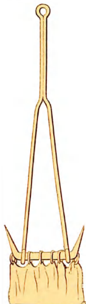
FIG. 49.—The End of the Dredge-Rope, showing the mode of attachment of the Bag.
