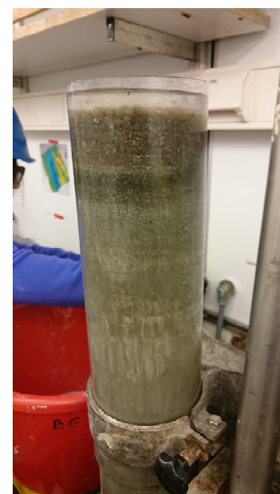
Multicore in the hydraulic slicer.
