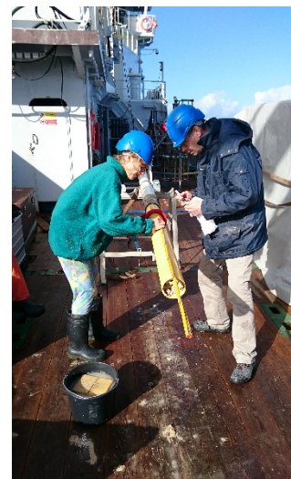
Cutting the piston core in 1 meter sections.
