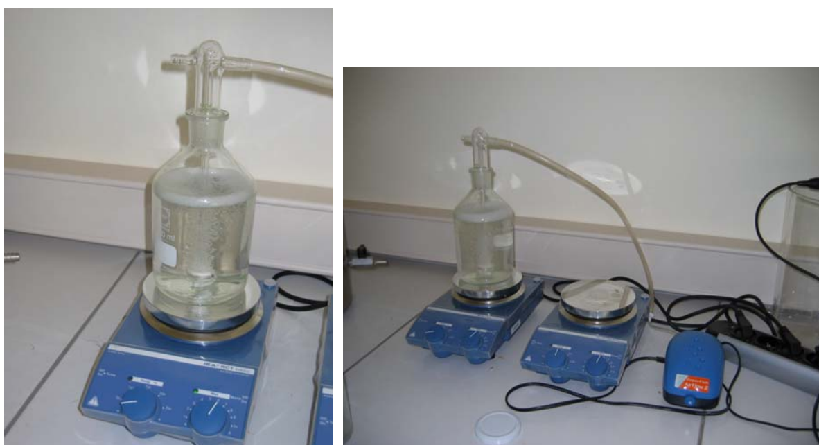
Figure 5. Photographs of the lab-scale stripping set-up for TBT-removal
