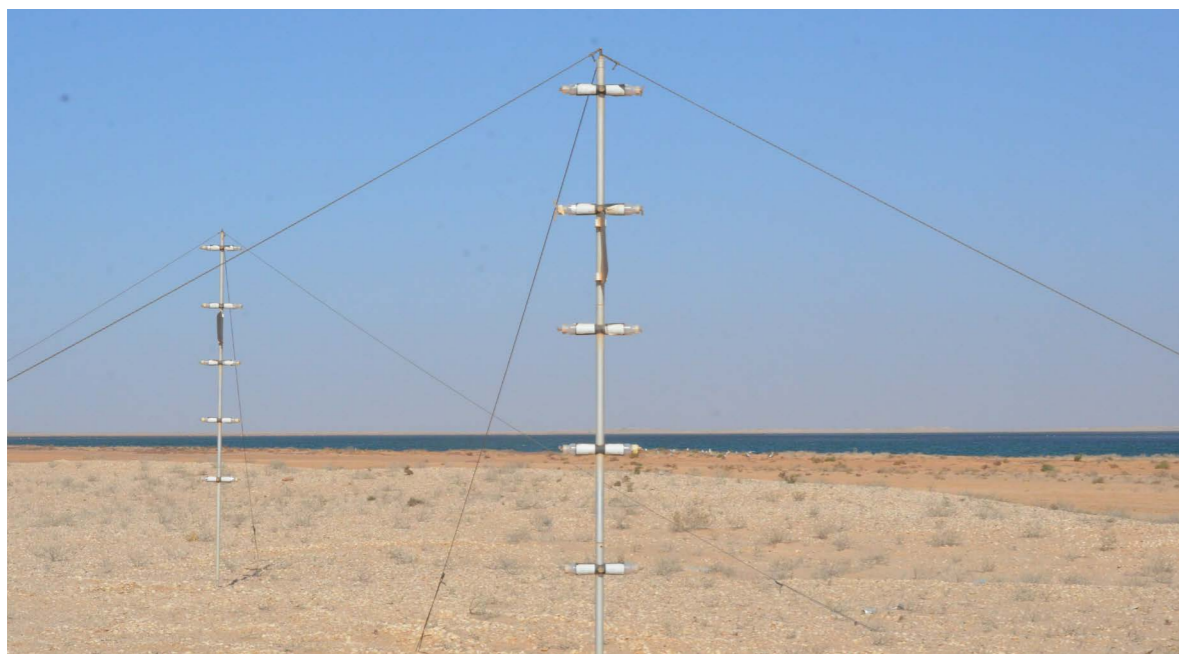
Fig 4.2: Dust sampling station in Iwik, Mauritanian coast. Two masts with MWAC samplers at 90, 140, 190, 240, and 290 cm above surface, sampling dust at a monthly resolution. A meteorological station monitors the meteorological conditions at the site, after which dust transport can be related to e.g., wind speed and direction (Friese et al., 2017)..(image by J. ten Horn)
