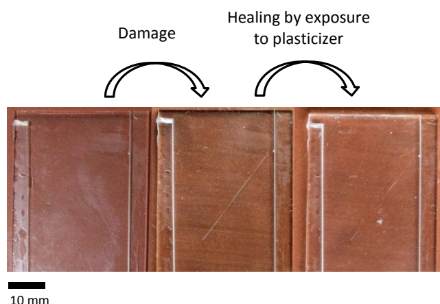
Figure 1. Example of an amorphous shape-recovery coating after scratching and recovery
