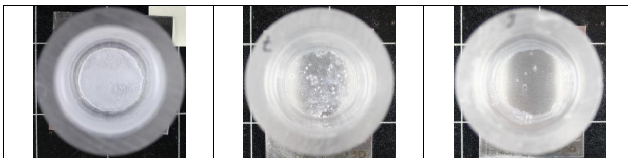
Figure 4: Photographs of samples immersed in NaCl 0.05M during 7 days; bare 2024 AA (left), 2024 AA covered with non impregnated mesoporous film (center) and 2024 AA covered with mesoporous film loaded with BTA (right).
