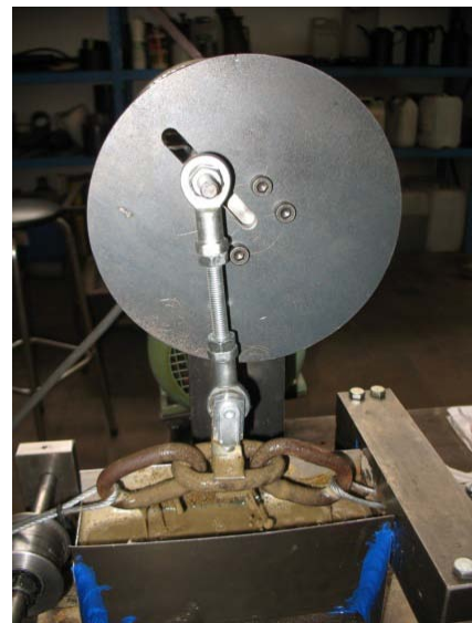
Figure 8: open chain cycle test rig developed at Laboratory Soete [8]
